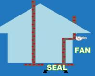
Some new homes are built with radon resistant construction. Or systems can be added to existing homes
